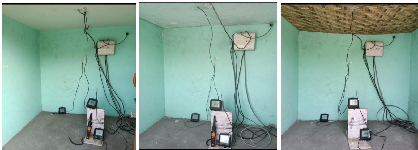
Figure 3.1– On Site images of Room with different insulation layer: (a) No insulation (b) Bamboo insulation (c) EPS
